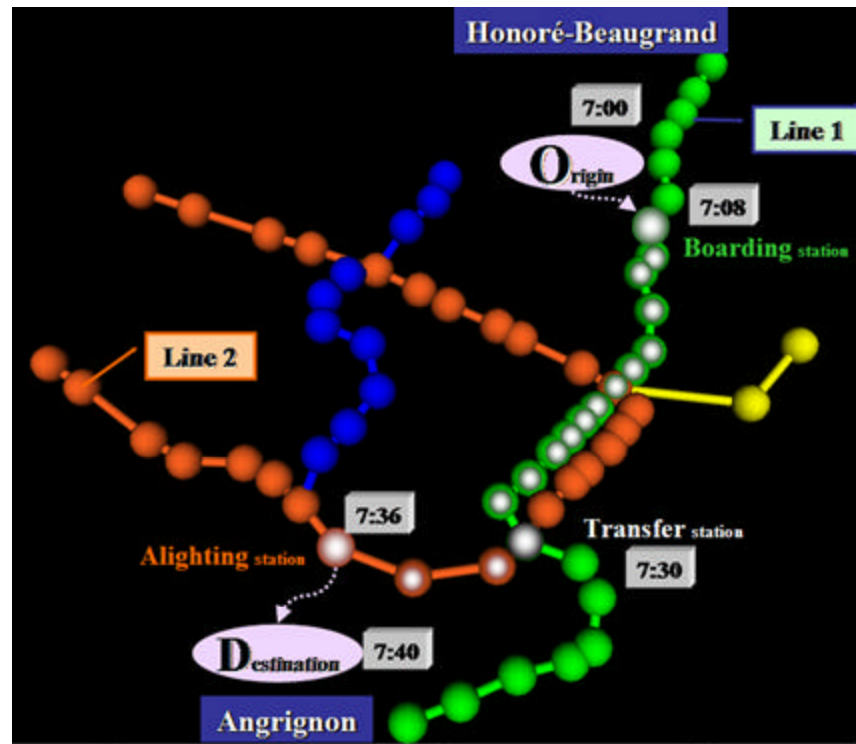
Figure 2 Example of trip and network elements considered in the processing of travel data: case of a single itinerary over the Montreal subway, in VRML.
