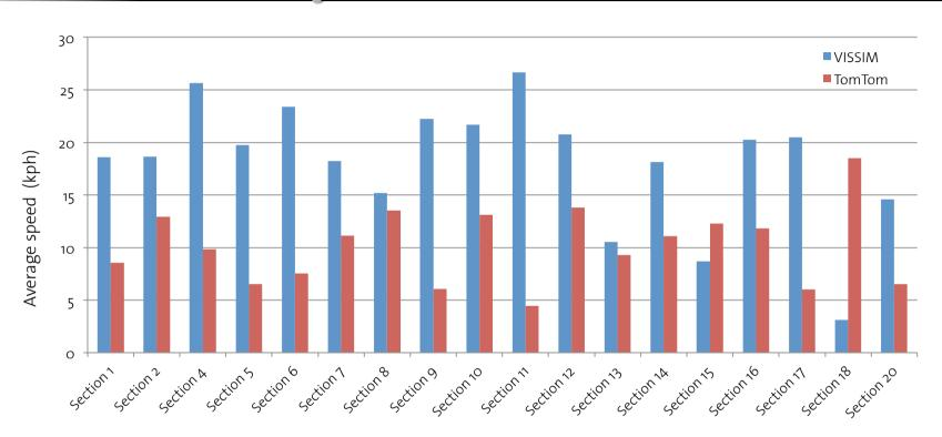
VISSIM consistently over-predicted the speeds in the network
