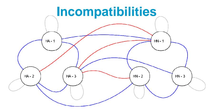
An <u>incompatibility graph</u> is introduced to model properly the situation. A compact representation is obtained by analyzing the graph connectivity.
