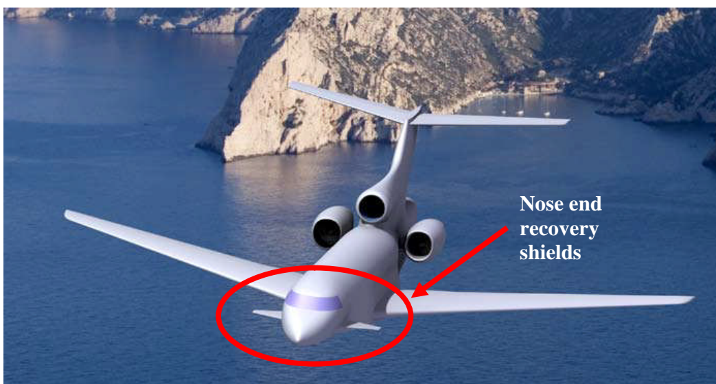
Figure 1. Recovery shields at the nose end of a T-tailed aircraft
