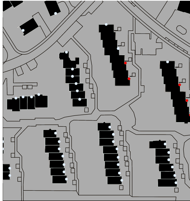
Example: Missing building separation
