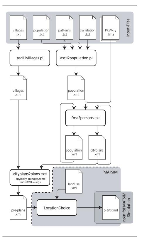
Figure 4: Data flow when using *fma2persons*
