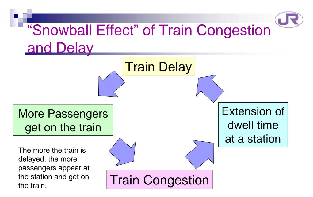
This effect is caused by dynamic interaction between passengers and trains.
